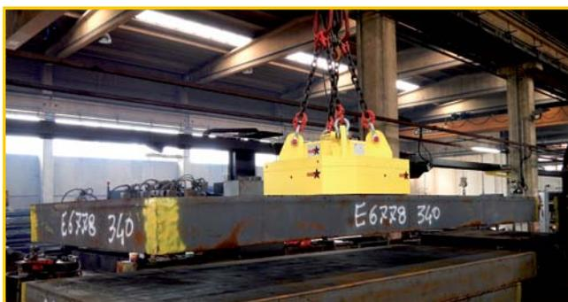
The well-structured SEP-modules, specially designed for the handling of slabs and forged blocks with an increased air-gap, are able to withstand high stresses and strains and are therefore extremely reliable over time.
