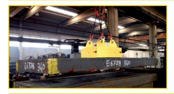
The well-structured SEP-modules, specially designed for the handling of slabs and forged blocks with an increased air-gap, are able to withstand high stresses and strains and are therefore extremely reliable over time.
